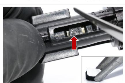
Fit the kit into the chamber, angle it so the tail inserts in the adjustment wheel first then adjust the bracket to the back of the chamber. Use Pin to lock
