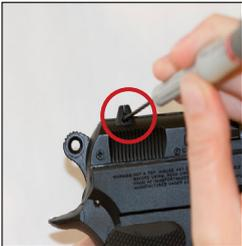
**Adjust the rear sight by turning the screw**
