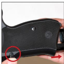
Push the Magazine release button and pull out the magazine.
